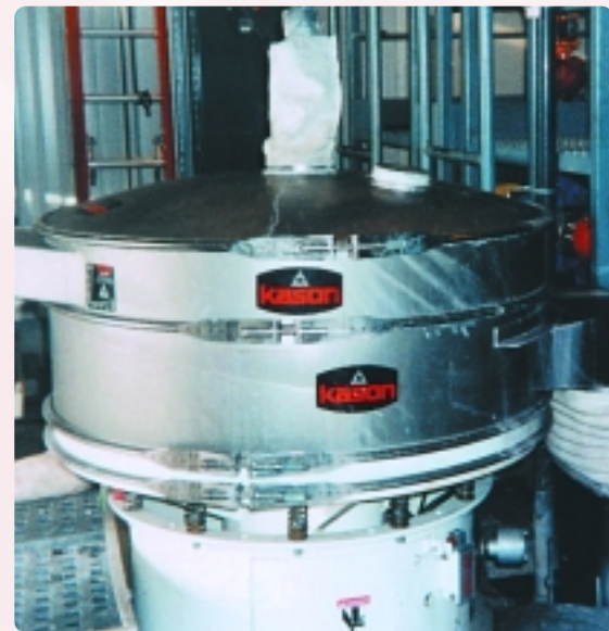
This stainless steel, 48-inch single deck, circular screen separator handles 158 gallons per minute of solids-laden waste.
