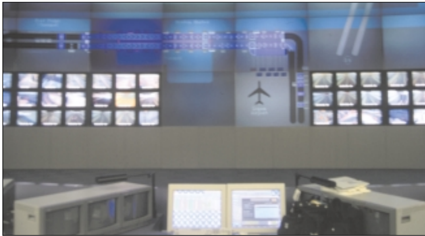
The Operations Control Center has two amphitheater rows of five workstations each facing a wall-sized rear-projection screen and a bank of 54 color monitors.
