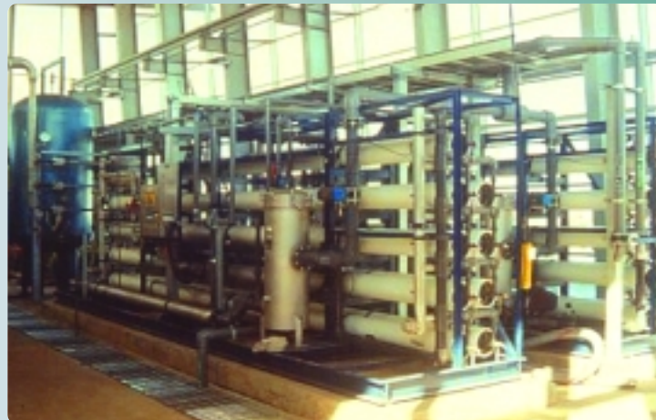
Left: The wastewater reclamation plant that recycled sewage and rainwater runoff at the Sydney Olympic Games Site in Homebush Bay, west of Sydney. The purification process involved the use of reverse osmosis (RO) technology.
