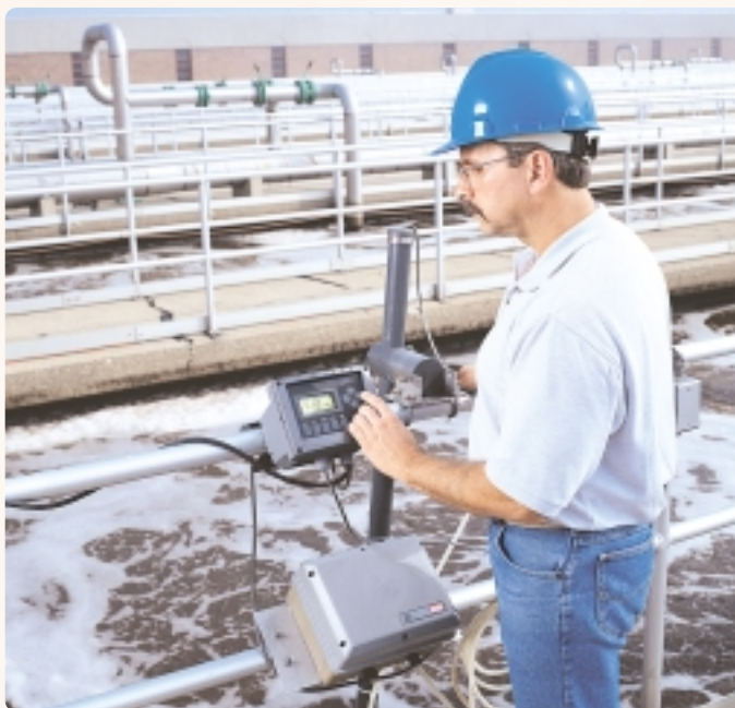
An operator calibrates a GLI self-cleaning D.O. system consisting of a Model D63 analyzer and a 5600-Series Ross Technology membrane cartridge sensor.
