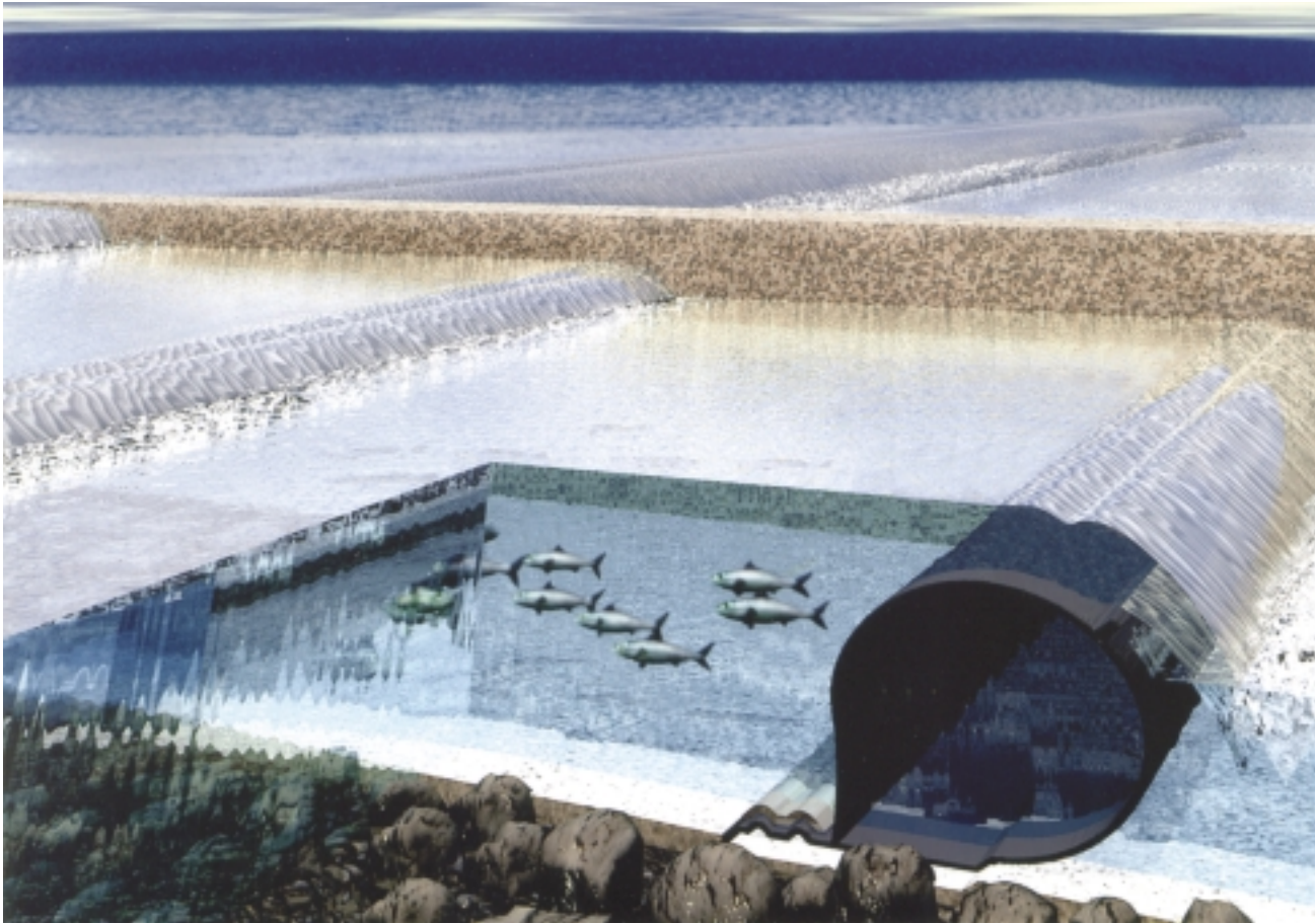
▲ Four water-filled rubber dams that stair-step in height from tailwater to headwater elevations would be used to enable migratory fish passage.
