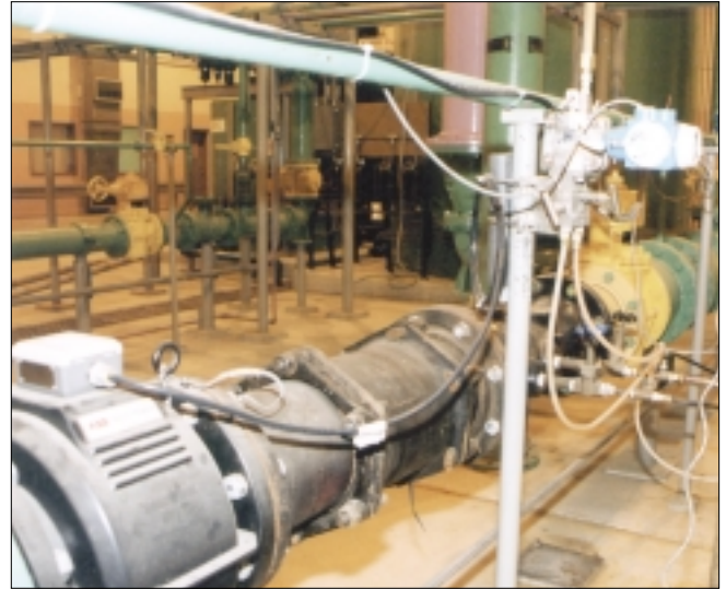
Figure 6: This test setup uses a MagMaster as the standard for verifying a Venturi tube primary element.
