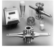
The Messenger liquid monitoring system features a compact transmitter and up to four sensors for process control, filter breakthrough and color measurement applications. Capable of monitoring turbidity. suspended solids and color simultaneously, this system can achieve a dynamic range of 0 to 1 ppm, 0 to 500 ppm or 100 to 10,000 ppm. Monitek, a Metrisa Co., Bedford, MA Write in 1195
