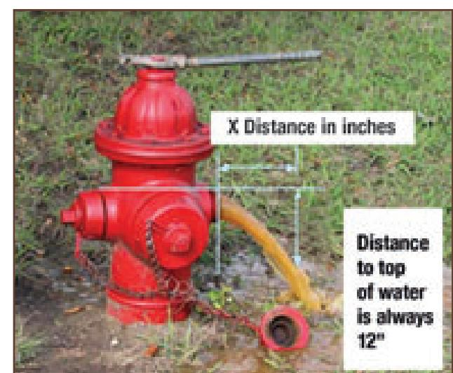
**Estimating flow from blow off valves and fire hydrants for flow ranges below 150 gpm in gpm**
