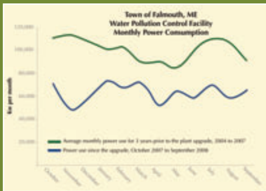
This graph shows the power consumption, measured by kilowatts per month, of the facility prior to the upgrade (green line) and after the upgrade (blue line).
