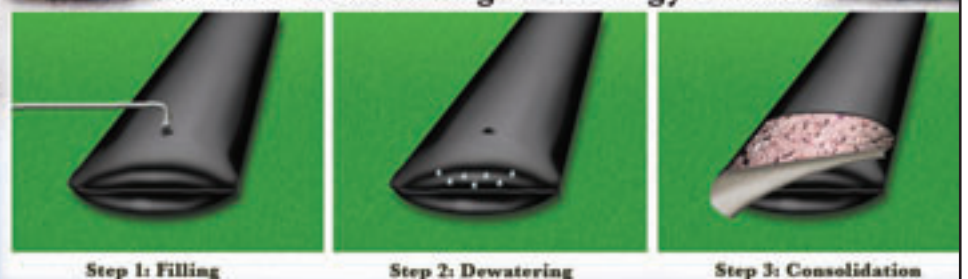
Geotube® Dewatering Technology Process
