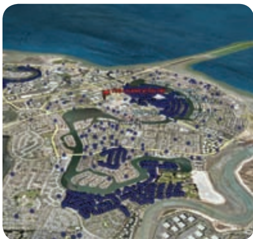
Foster City replaced its 4-sq-mile service area's outdated meters with a two-way AMI fixed network.
