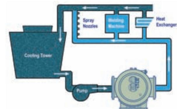
**1** Cooling towers are virtual vacuum cleaners for air- and water-borne particulate that can foul valuable downstream equipment such as spray nozzles, welding operations, chillers, heat exchangers and small bore piping. Unlike side-stream filters sometimes used with cooling towers, the full-stream use of a multi-element strainer enables cooling systems to remain online continuously.
