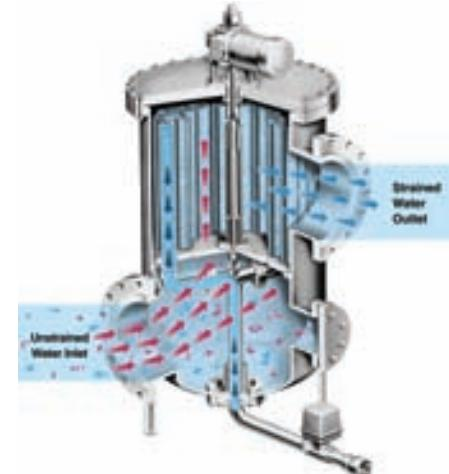
**3** Multi-element self-cleaning strainers provide continuous full-stream protection with minimal backwashing or maintenance. Although multi-element strainers may be used in a side-stream application, full-stream configuration is normally recommended because it provides complete filtration at all times.
