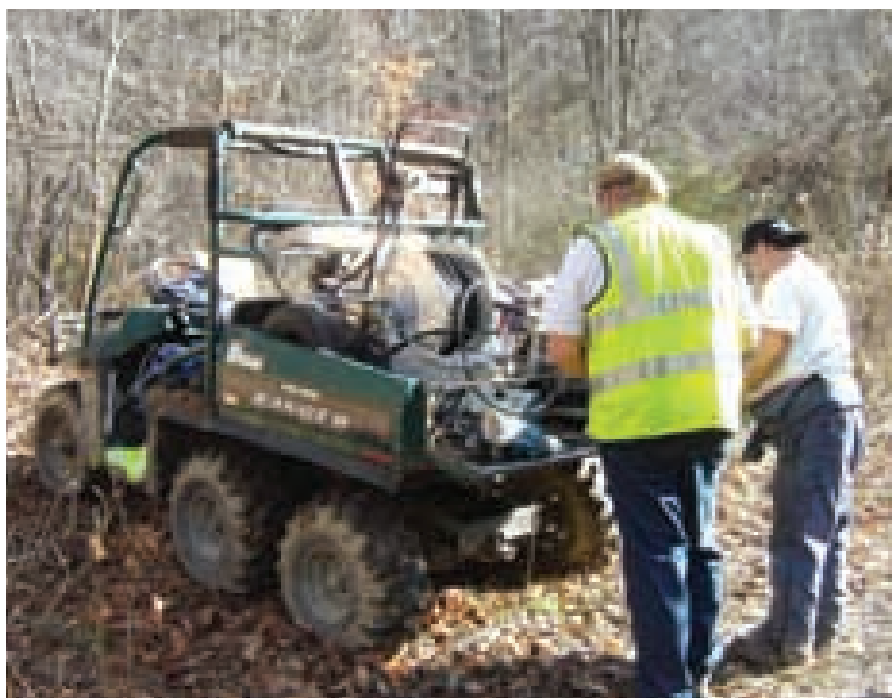
The Solo robot inspects without an operator present, collects 360-degree spherical video and has portable off-road abilities, making it ideal for off-the-grid inspection of 8- to 12-in. pipe.
