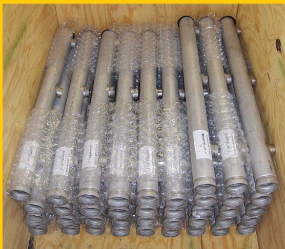
These assemblies are modular and can be shipped economically via common transport. The units are field-assembled easily using vitaulic coupled connections.
