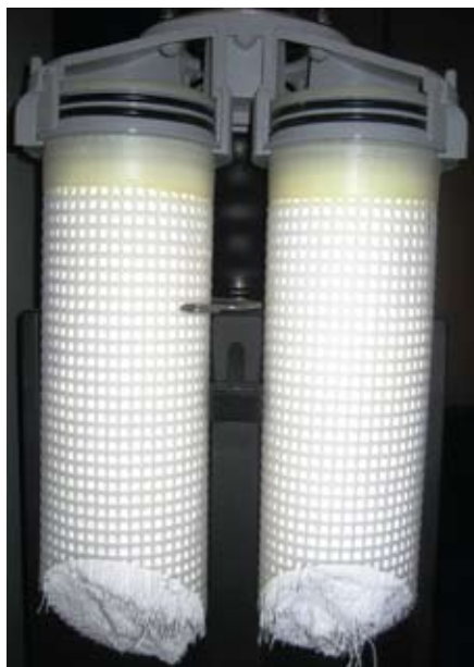
Polypropylene membranes, each containing 15,000 fibers with a nominal pore size of 0.20 microns.
