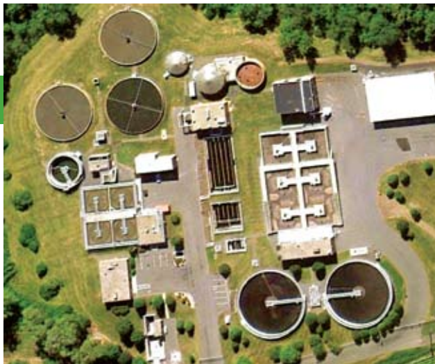
A WWTP in Farmington, Conn., decreased effluent TN 14% over 10 months of treatment.
