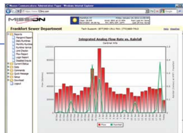
SCADA is deployed at Frankfort for the city's flood station control systems.
