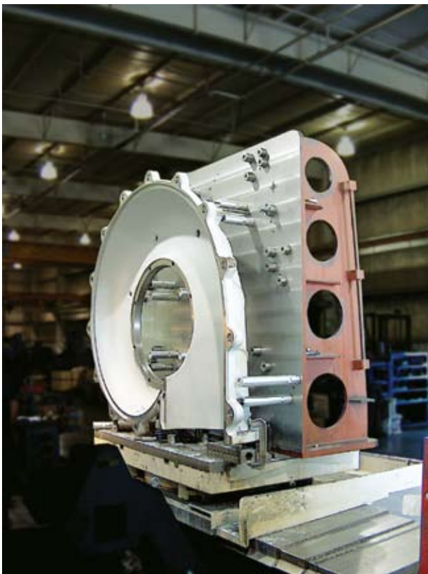
The slurry pump housing half-mounted on the fixture, situated on a horizontal boring mill.
