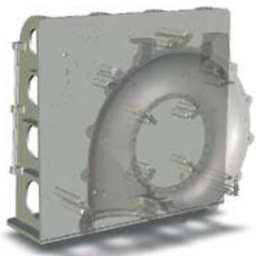
CAD models of the two halves of the slurry pump housing on the dedicated fixture.
