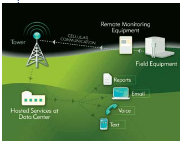
Information is transmitted from remote and unmanned equipment into a data center.
