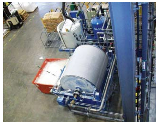
The Auto-Vac is prepped, prewired and skid mounted for easy installation.
