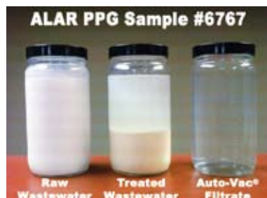
Chemical separation is necessary to break emulsion and precipitate metals.
