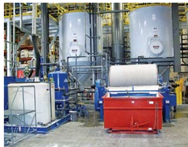
PPG uses a series of three tanks: equalization/holding, chemical batch treatment and clean water filtrate (dilution) tanks. The Auto-Vac is capable of filtering 12,000 gal per day of PPG's latex wash water and wastewater (after dilution).
