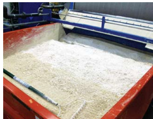
The Auto-Vac separates the solids from the liquids, producing a dry cake that has the consistency of damp sand. Dry solids typically measure greater than 45% raw solid content by weight.
