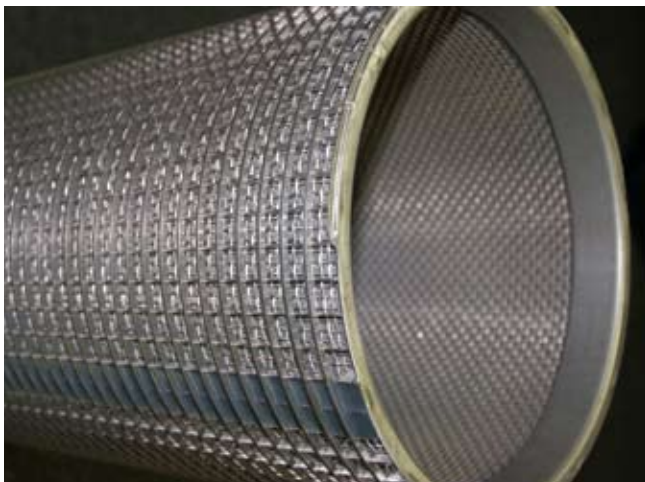
Four layers of stainless steel screen provide filtration down to 10 microns to protect membranes from sediment and biofouling.
