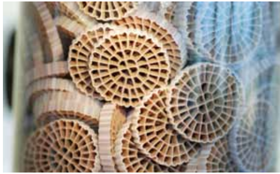
Biofilm carrier elements form the basis of the IFAS process.
