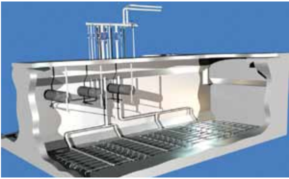
A cutaway illustration of a HYBAS system reactor tank.
