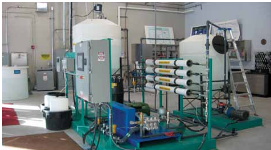
Batch-scale seawater RO system at CHIWAHA lab of El Paso Water Utilities
