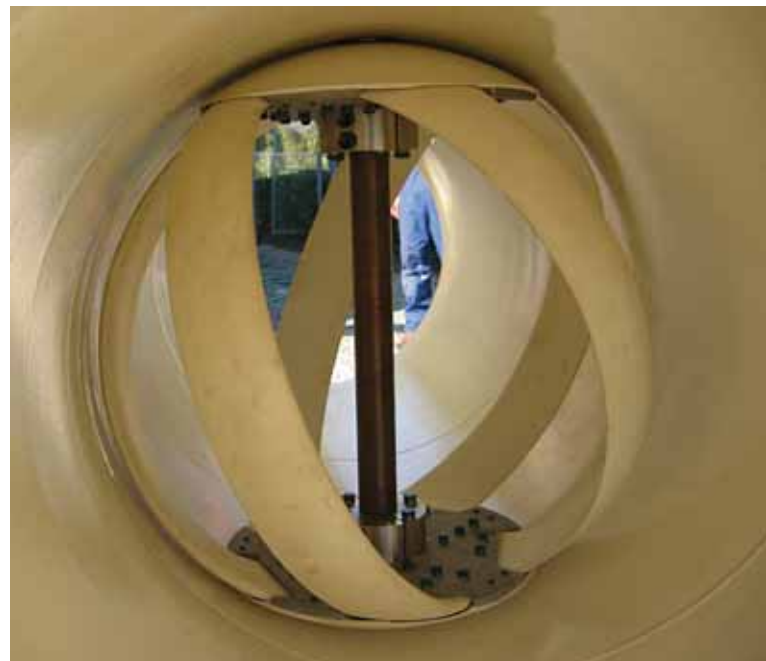
The in-pipe turbine in this system harvests energy without disrupting pipeline operations.
