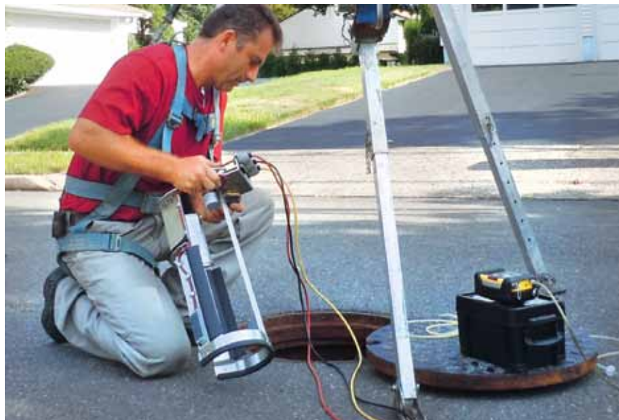
NIST traceable billing meter monitors flow from neighboring communities.
