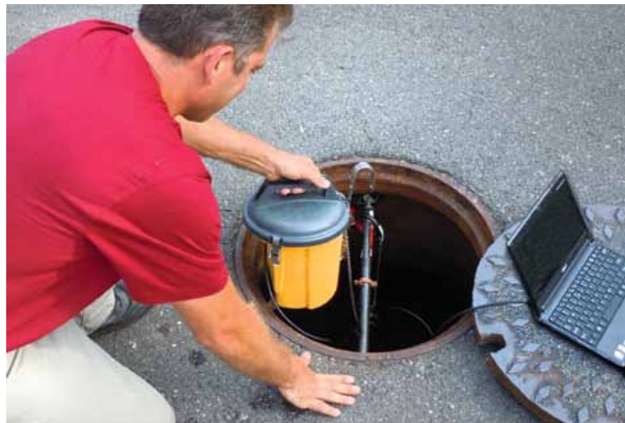
An I&I detection monitor becomes fully operational in 15 minutes without confined-space entry.
