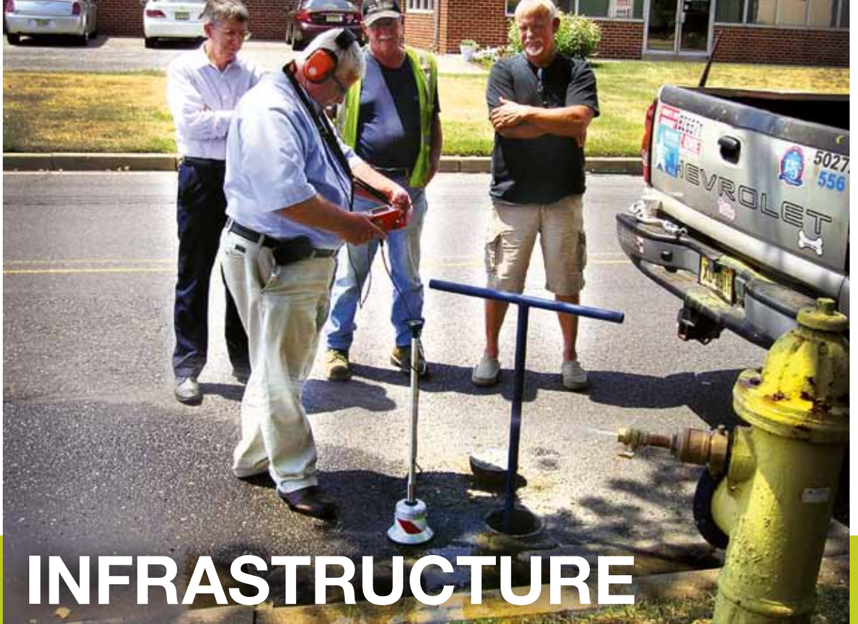
Leak detection vendor Jim Fay demonstrates the use of an acoustic monitor with a ground microphone to training attendees and instructor Dave Hughes. The small jet of water coming from the hydrant generates an audible leak noise.
