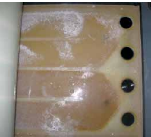
Scaling problem on anion exchange membrane
