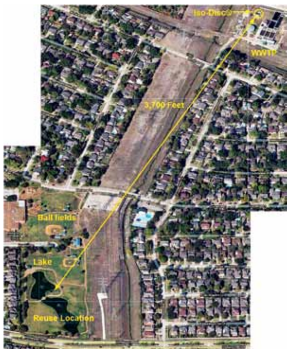
The filtration system is located at the wastewater treatment plant, 3,700 ft away from the reuse location.
