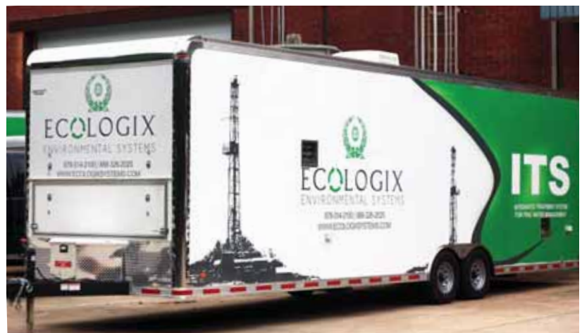
Below: The mobile chemical treatment unit prepares the water for physical separation.
