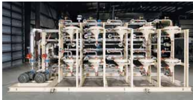
The produced water filter skid featured an earlier version of the Tequatic Plus fine particle filter.
