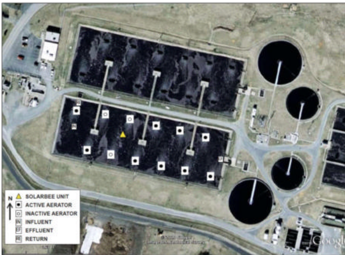
Figure 1. An aerial photograph of the Eden, NC, Mebane Bridge WWTP, and symbols in the South Basin as indicated in the key. The return (RE) indicates the return of activated sludge from the clarifier basins shown on the right.
