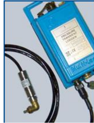
Figure 11: Example of a pressure transient logger
