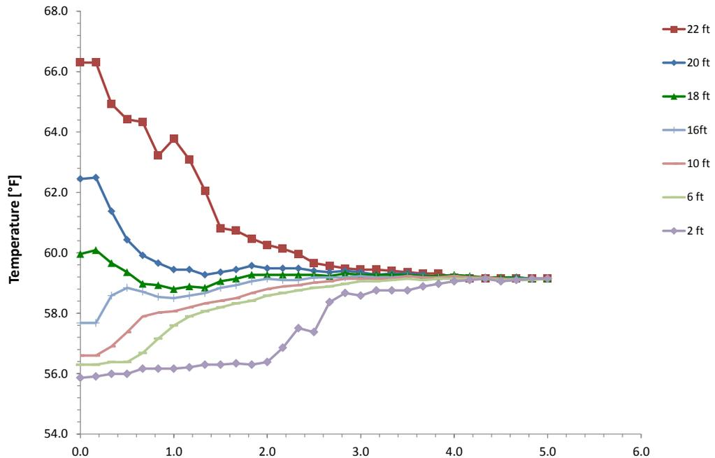
**Figure 1.** Data from the PAX Water Mixer in a 500,000-gal tank shows that the water temperature at each level converged within 4 hours.
