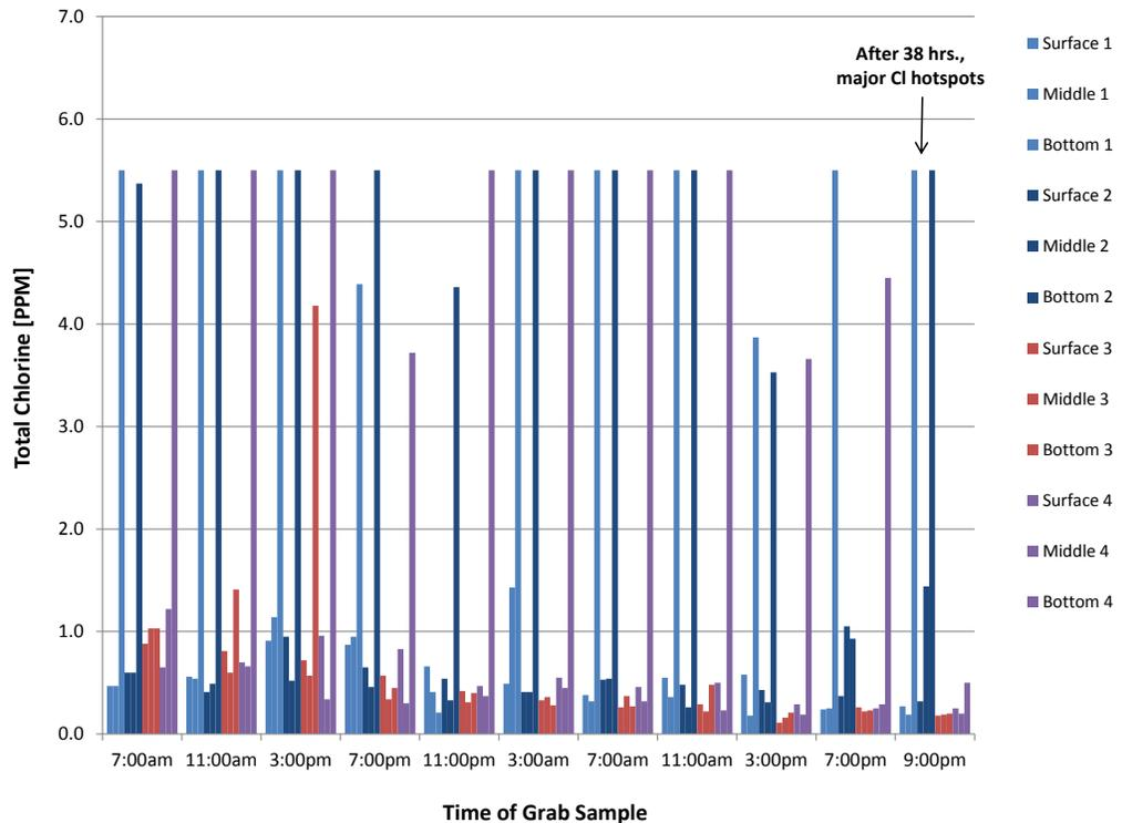
**Figure 5.** Data from a cheaper submersible mixing system in a 4MG tank dosed with 50 gallons of hypochlorite shows that water chemistry never became uniform, even after 38 hrs. of mixer operation.
