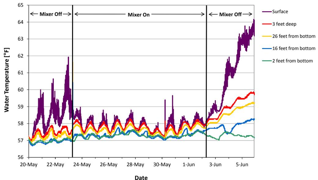
**Figure 2.** Data from the PAX Water Mixer in a 4MG tank shows that the water temperatures became uniform within 0.5 °F. When the mixer was turned off, the tank quickly became thermally stratified.
