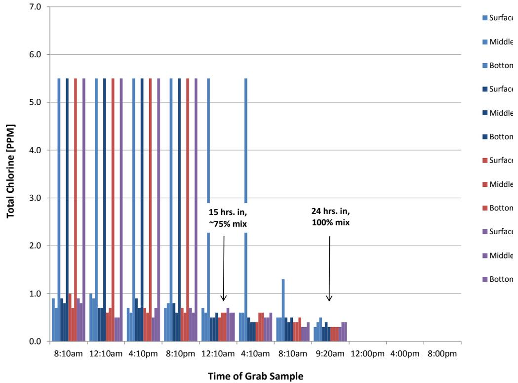
**Figure 4.** Data from the PAX Water Mixer in a 4MG tank dosed with 50 gallons of hypochlorite shows that water chemistry became uniform within 24 hrs.
