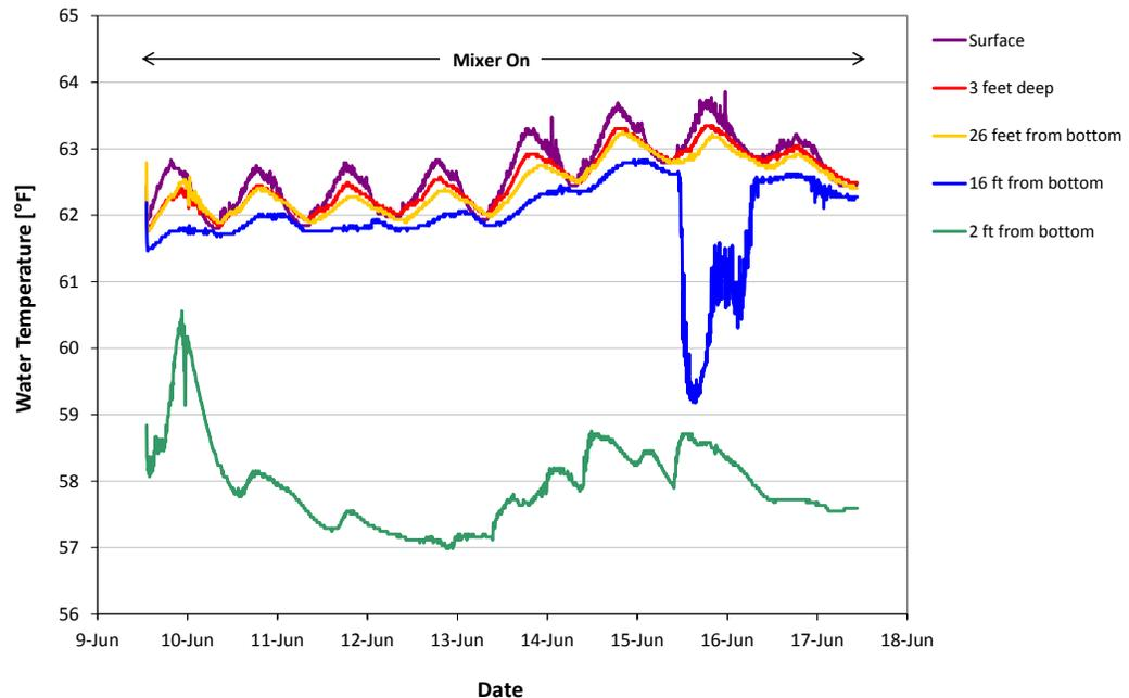
**Figure 3.** Data from a floating mixing system in a 4MG tank shows that the mixer was unable to eliminate thermal stratification. A 5 °F temperature difference between the upper and lower water layers persisted.
