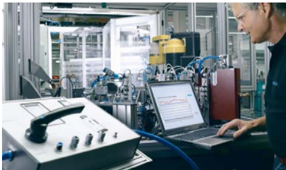
Figure 10: Measurement of compressed air consumption
