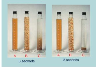
ACTIFLO Softening is designed to reduce Hardness, Alkalinity, Silica and Heavy Metals by addition of lime and/or Soda Ash.
