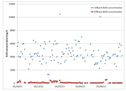
Figure 7: Influent and effluent BOD concentrations for the AnMBR system at the confectionery manufacturing plant
