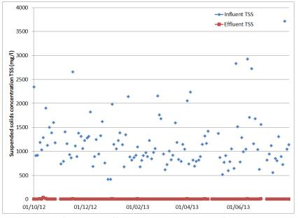
Figure 8: Influent and effluent TSS concentrations for the AnMBR system at the confectionery manufacturing plant
