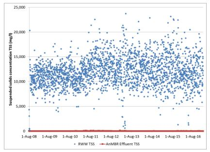
Figure 4: Influent and effluent TSS concentrations for the AnMBR system at Ken's Foods
