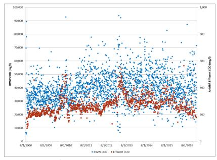
Figure 3: Influent and effluent COD concentrations for the AnMBR system at Ken's Foods
