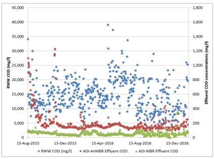
Figure 12: Raw wastewater and effluent COD concentrations for the AnMBR + MBR system at Kellogg Company's Pikeville Plant
