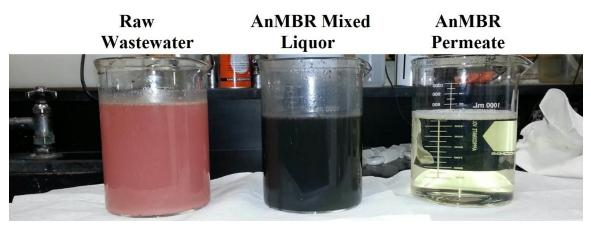
Figure 9: AnMBR influent, mixed liquor, and permeate at the confectionery manufacturing plant
