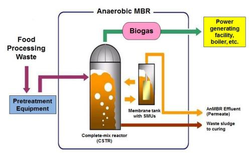
Figure 1: General process flow diagram of the AnMBR process
