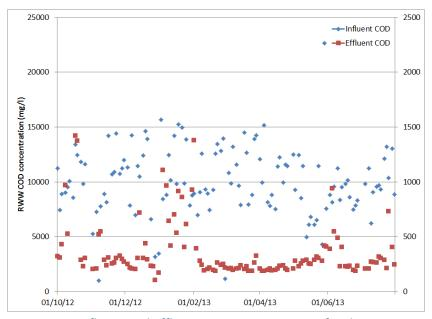
Figure 6: Influent and Effluent COD concentrations for the AnMBR system at the confectionery manufacturing plant
