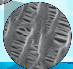
Hydrophobic membrane with pores approx. 0.03 \mu\text{m}
