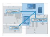
Modular automation means that every module is equipped with a dedicated terminal CPX together with a valve terminal and controller. 4
