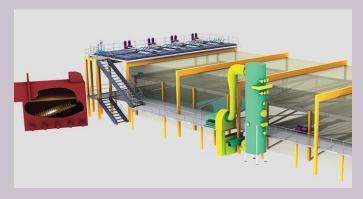
**BioCon™ ERS** (Energy Recovery System) is a safe and sustainable drying and combustion system that combines the efficiencies of a convective air low temperature belt dryer with a biomass furnace to recover sensible heat and combust all organic material, including PFAS compounds.
